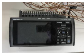
Fig.6 Left: Thermocouple Right: Date logger
