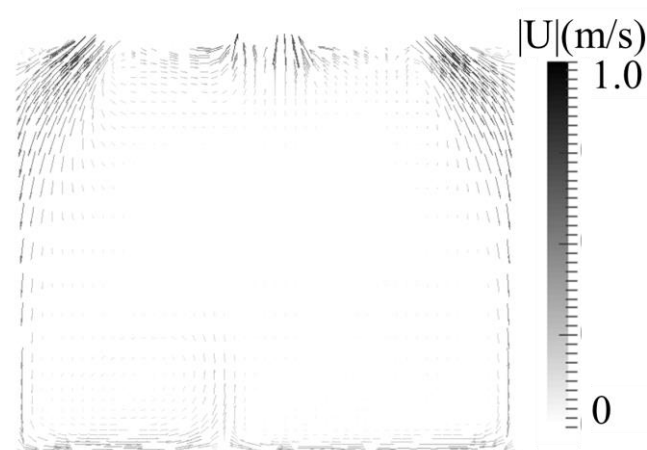
Fig. 9 Wind speed distribution at central section of the room (no-radiant)
