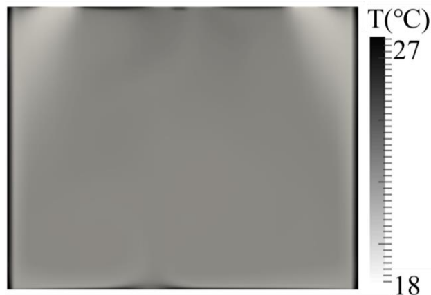
Fig. 7 Temperature distribution at central section of the room (no-radiant)
