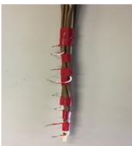
Fig.6 Left: Thermocouple Right: Date logger
