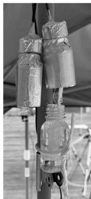
Fig.1 TC sensor with radiation shield.
